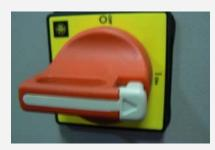
2. Switch on the safety circuit of the band saw (button **2** – control panel of the band saw).
