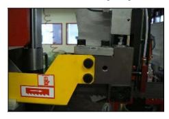
Never switch on the saw band driver if this cover is not mounted!
