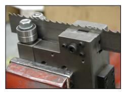
15. Using a short piece of the blade used on the machine, adjust the width of the gap between the guides. Loosen the central screw. Set the gap by central adjusting screw. Belt guides must walk freely without large and will also not scrub.
