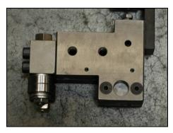
22. Insert fixed hardmetal guiding and mount hard metal with two screws.
