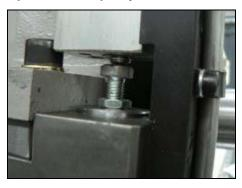
The lower stop limits the lowest position of the saw arm. This stop point has to be checked at least once a month. If the lower stop point is wrongly adjusted, the cutting table can be deeply cut or the material will not be cut completely.
