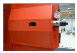
• Tighten the saw band by means of the TENZOMAT on the optimal value (table is on the Tenzomat).
