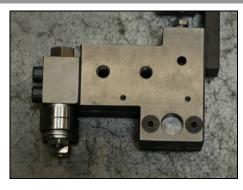
14. Insert fixed hardmetal guiding and mount hard metal with two screws.
