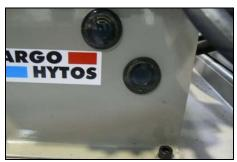
Pull up the gauge and check the state of the oil. The oil level must be situated between water-glas.
