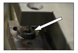
17. Insert the disc springs. The number of disc springs must match the number of dismantled springs. Disc springs are folded against each other 1 to 1 Odd plate spring is near the harmetal carbide.
