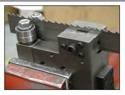
23. Using a short piece of the blade used on the machine, adjust the width of the gap between the guides. Loosen the central screw. Set the gap by central adjusting screw. Belt guides must walk freely without large and will also not scrub.
