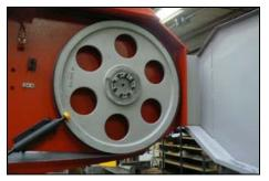
The band saw is stated to the operation, when the covers is closed!
