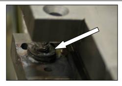
9. The number of disc springs must match the number of dismantled springs. Disc springs are folded against each other 1 to 1 Odd plate spring is near the harmetal carbide.
