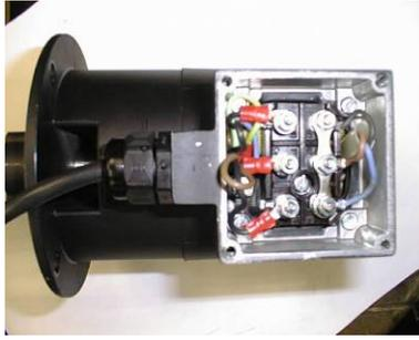
3. Remove the cover of the pump terminal switchboard. Disconnect 4 terminal connectors of the input cables. Cables are identified according to the red clamps..
