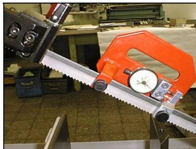
3. Stretch the saw band until it is stretched to the recommended value
