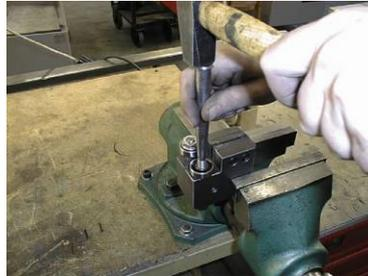
7. Install eccentrics to the cubes. Install components on both eccentrics in given order. Put bearings by means of the preparation on eccentrics.
