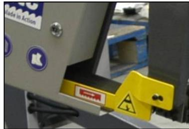
6. Install the yellow protective cover of the band. The arrow on the cover must match the direction of the arrow on the band. If it does not, you must turn the band round.
