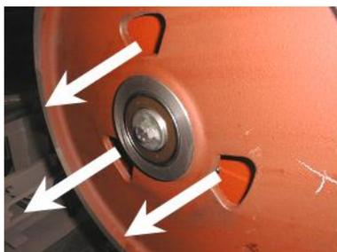
3. Pull off the wheel from the shaft by means of the three-armed puller. If bearing stayed on the shaft, pull off it too
