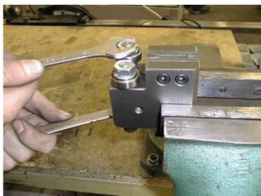
3. Tighten the guiding cube to the vice and dismantle both eccentrics with bearings following way.
