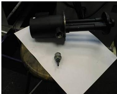
6. Screw on the cable bushing and cover of the terminal block. Do not forget the rubber gasket! Tighten the cooling liquid hose with non-stick tape and screw it again. Install cooling liquid hose, place the pump on the sheet metal holder and screw it
