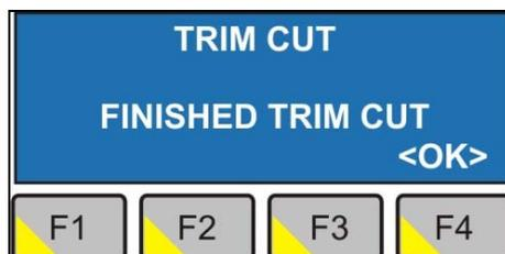
4. If the operator chose the trim cut on LCD is info about the progress. After the completion of trim cut, confirm by button F4.
