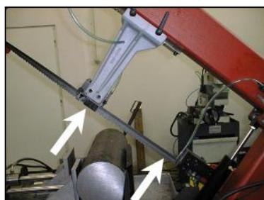
2. Insert new saw band in the guide cubes. Make sure the saw band runs between both guide rollers and it is pushed all the way to the top.
