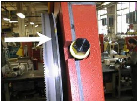
4. Check saw band placing on the wheels.
