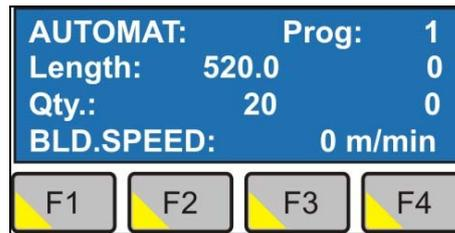
6. The operator is informed about the automatic cycle on the LCD.
