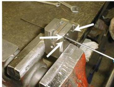
2. Loosen the adjusting screws of the metal guide.
