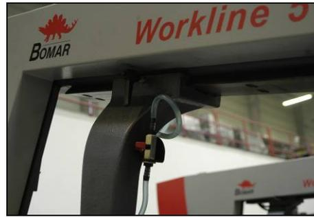
1. Release the stopping lever of the listel. Move the left part of the guide so that the left edge of the guide blocks is as close as possible cutted material.
