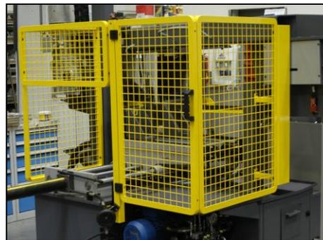
The doors of the protective fencing are protected by limit switches. If the limit switch is open, the machine is turned off.
