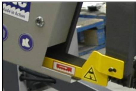
Never switch on the saw band driver if this cover is not mounted!
