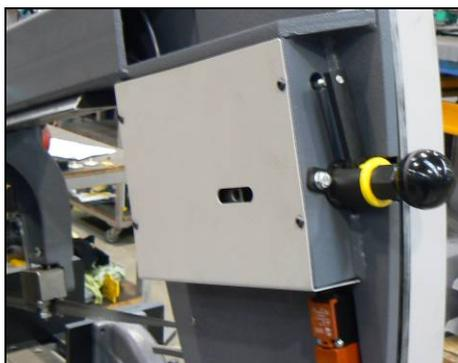
The saw band run is set with screw in the stretching cube on the saw frame. Optimal distance has been determined at **1 – 3 mm**.
