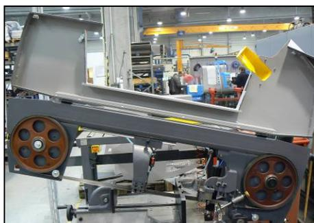
**The band saw is stated to the operation, when the covers is closed!** Limit switched on saw arm control if covers are open or not.
