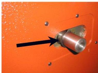
5. Clean the shaft and grease it with oil. Insert retaining ring to the groove.
