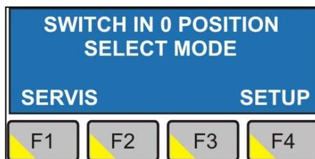
Parameters in the menu SERVICE are password protected. The parameters in the SETUP menu are common and are not password protected.
