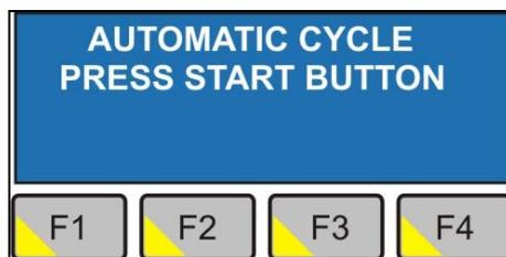
5. Now begins the automatic cycle. It begins by pressing the START button. The work cycle begins on the program, where was editing completed by button F3 (END) and ends on the last non-zero program. Example: I edited program no. 2 last time (F3 was pushed on program no.2), program no. 3 and 4 has correct values, programs no. 5, and more are empty. Control system loads program no. 2 then program no. 3 and last performed program is no. 4.
