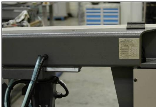
Machine label is placed on saw frame.
