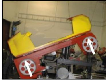
3. Put the saw band on both guide wheels. Make sure that the saw band ridge fits tightly to the wheel rim. Then push the saw band as far back as possible.
