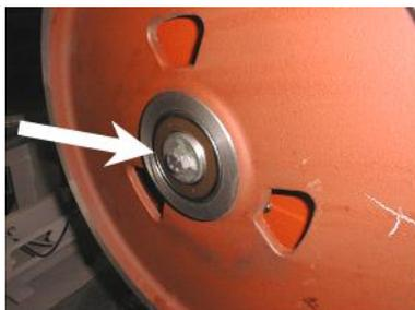
2. Screw off the screw and take down the washer.
