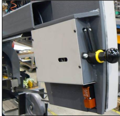
The device contains limit switch. Check the stretching carefully and periodically – eventually adjust.
