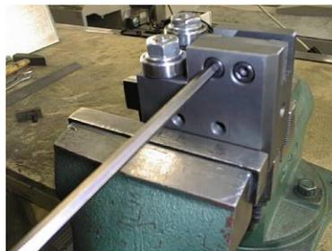
4. Loosen the binding screw of second metal guide. Remove the hard metal guide
