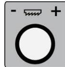
Use the frequency convertor on control panel (pos. 6) to adjust requested speed of the saw band.
