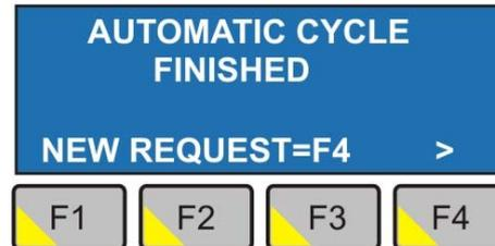
7. After completing automatic cycle, operator may enter new values for the next cycle (F4).
