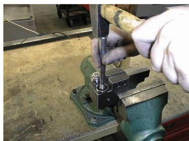
5. Remove eccentrics from bearings by means of the swager
