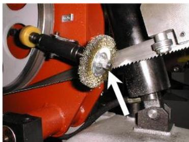
1. Release the nut of the brush, exchange old brush to new brush and screw on the nut of the brush.
