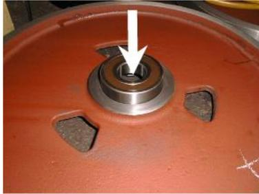
8. Insert the bearing to the hole in the wheel and press it to the retaining ring.
