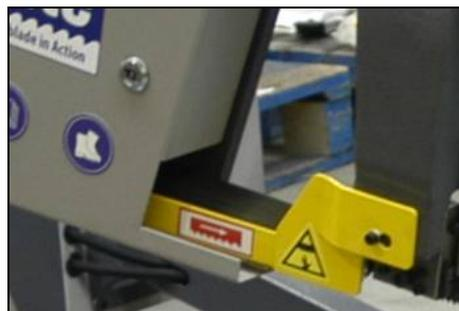
After the machine has been successfully connected, briefly switch on the machine and put the driving engine of the band in the running position. The direction must be in accordance with the arrow direction on the saw band cover. In case the direction of the saw band does not match, two phases at the terminal strip must be switched.
