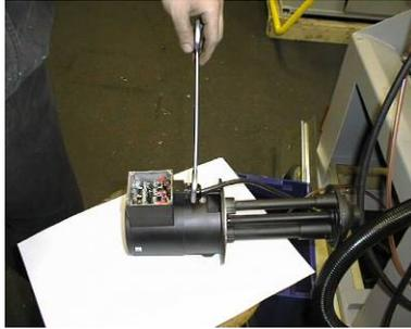
4. Loosen the bushing and pull the cable out from the pump.
