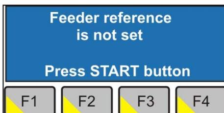
Operator is informed that the machine is not referred after machine start. For machine referring switch into automatic mode. Then START button begin flash. Press START button for begin referring process. After this process press F4 to confirm.
